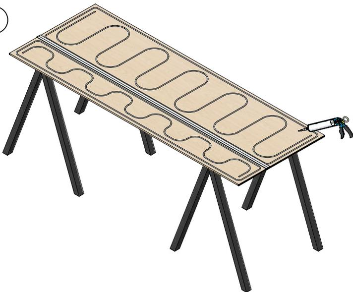
9. Glue the back side of the wall panels using our grab adhesive.
