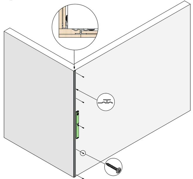
2. When installing an outer corner with a finishing strip, you start by installing a joint profile. Make sure that you go over the edge enough to cover both the wall panel and the gap before screwing on the SKARV profile and that it is straight.
