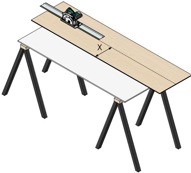
7. Saw the last wall panel at the correct width using a circular saw or a shadow gap saw.
