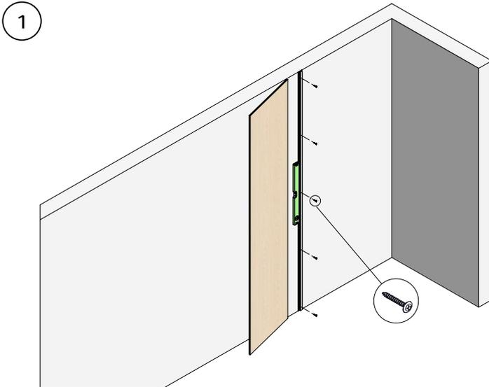
1. Screw our aluminium JOINT profile into place. Make sure the profile is level by using a spirit level.
