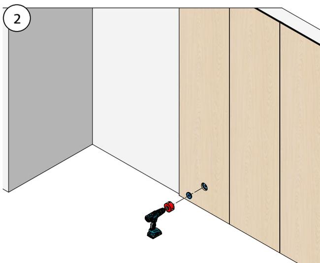
**2.** Then install the wall panel over the electric switch/plug socket/spotlights. Place the detector there so you can find where to drill the hole. Drill using a hole saw drill bit.
