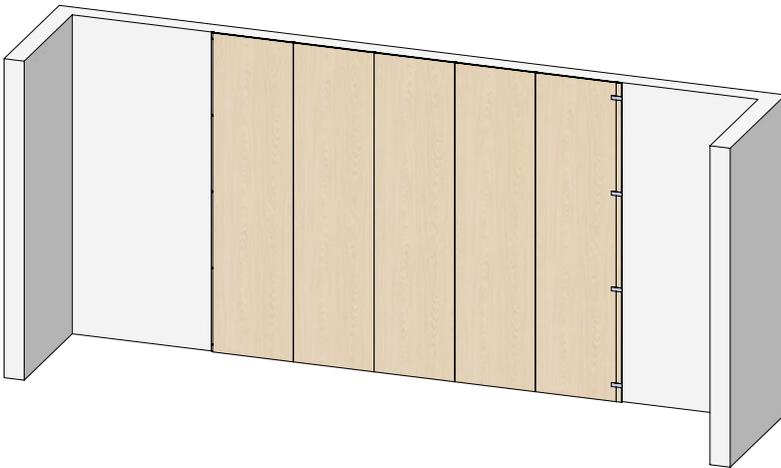
4. Install the remaining wall panels in the same way using our JOINT profile.
