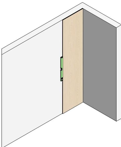
3. Insert the wall panel in the START profile. Double check that the wall panels are level using a spirit level.
