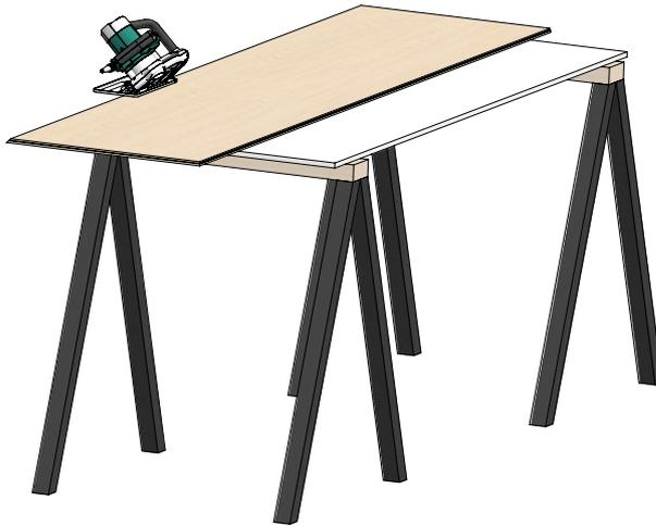
1. Installing outer corners. Mitre together the edges of two wall panels in the outer corner.
