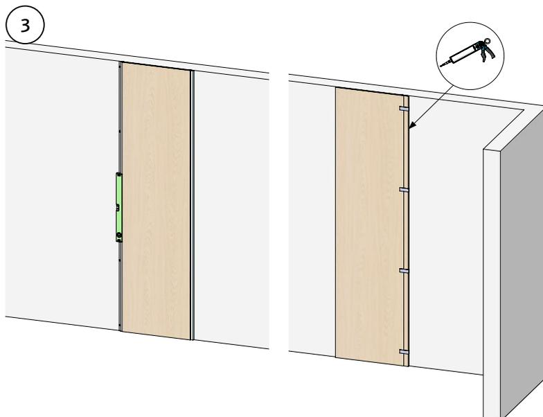
3. Place our grab adhesive on the end strip. Insert it into our JOINT profile. Tape so that it is firmly placed against our wall panel and allow the glue to cure.
