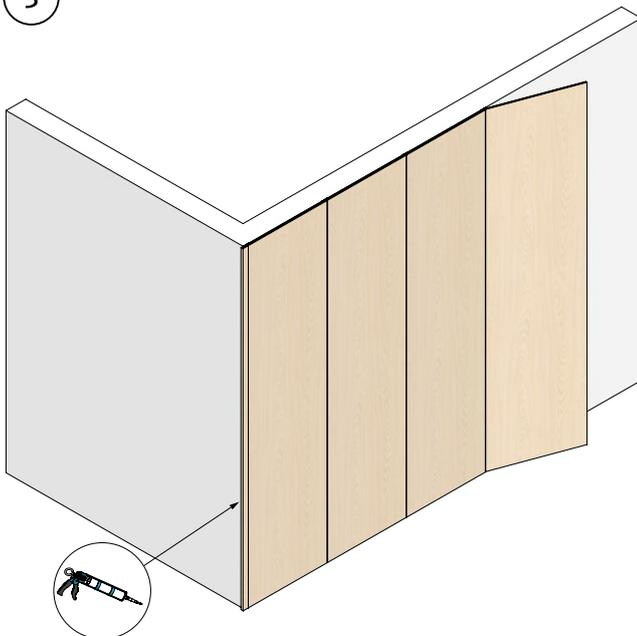
3. Glue with our mounting adhesive on the finishing strip. Insert it into our SKARV profile. Tape it against our wall panel and let the glue harden. You can continue installing that wall while the glue cures.
