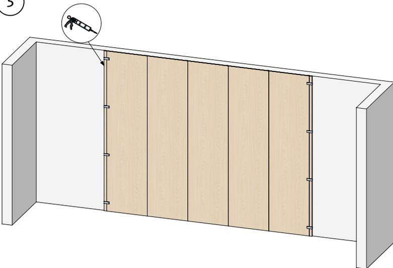
5. Place our grab adhesive on the end strip. Insert it into our JOINT profile. Tape so that it is firmly placed against our wall panel and allow the glue to cure.
