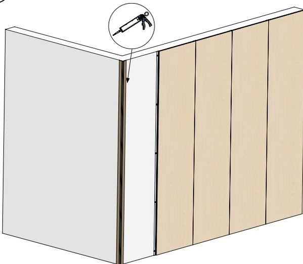
3. Screw or glue our SPACER strip into place before installing our wall panels so that the distance between our wall panel and the wall will be correct.
