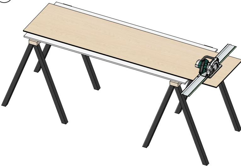
1. Measure the height of the existing wall. Saw the wall panel at the correct height using a circular saw or a shadow gap saw
