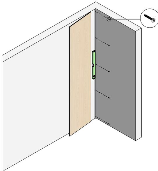
2. When installing between two existing walls, begin by screwing our START profile in place. Make sure the profile is level by using a spirit level. Screw the profile into place keeping 50 mm from the upper edge and the lower edge, then evenly distribute the profiles in-between.
