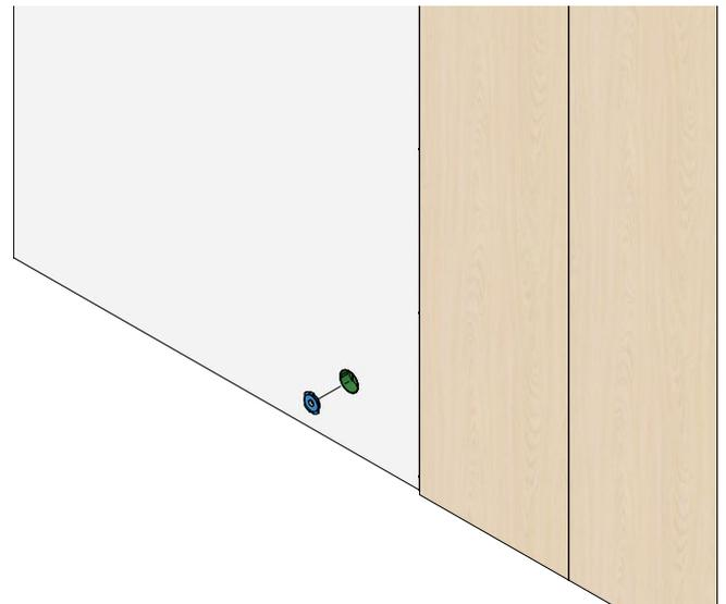
**1.** Externally mounted Electric switch/Plug socket/Spotlights Remove the electrical socket cover and fit a junction box insert.
